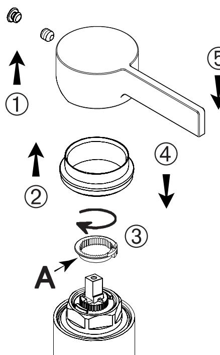
**GB** A temperature-control ring (**A**) attached to the valve will control leftward lever movement and thus adjust the temperature of hot and cold water (according to ①②③④⑤)
